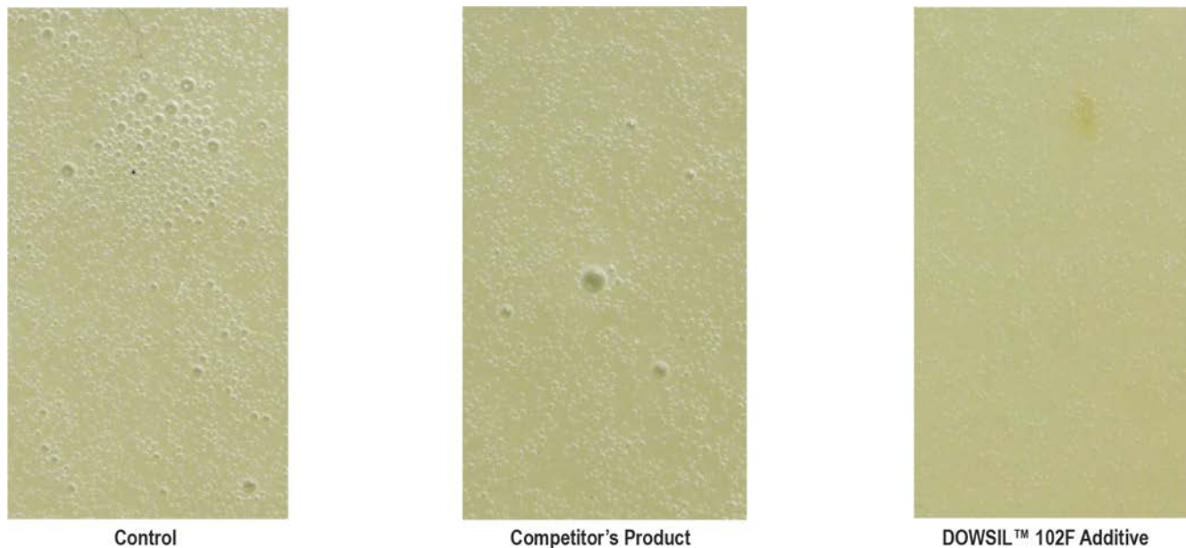
Figure 2: DOWSIL 102F Additive at 0.4 weight % as supplied in epoxy protective base coat with crosslinker and thinner inside. After shearing 15 minutes at 1500 RPM with dissolver blade, pour the same quantity of paint into flat container and wait for curing. Surface appearance after curing shows that DOWSIL 102F Additive is more effective at controlling foam than competitive products, indicated by less bubbles left on the surface when using DOWSIL 102F Additive.
